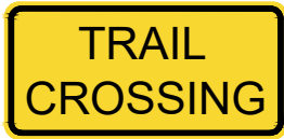
TYPICAL PTH 3 BICYCLE TRAIL CROSSING LEFT TURN STREET SIGN (WC-44L + WC-44T)
