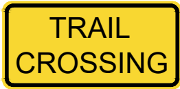
TYPICAL PTH 3 BICYCLE TRAIL CROSSING RIGHT TURN SIGN (WC-44R + WC-44T)
